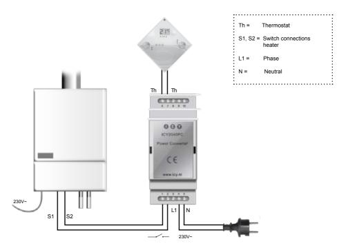
The Power Converter is connected to the normal connection that is already present between the heater and the room thermostat.
